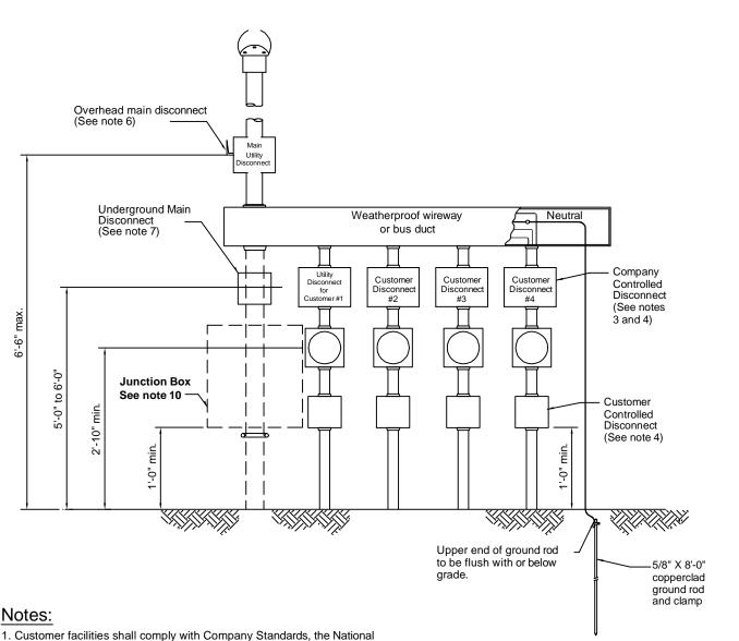
1. Customer facilities shall comply with Company Standards, the National Electrical Code, and authorities having jurisdiction. All material shall be suitable for outdoor use. Equipment to be installed at a location designated by the Company.
